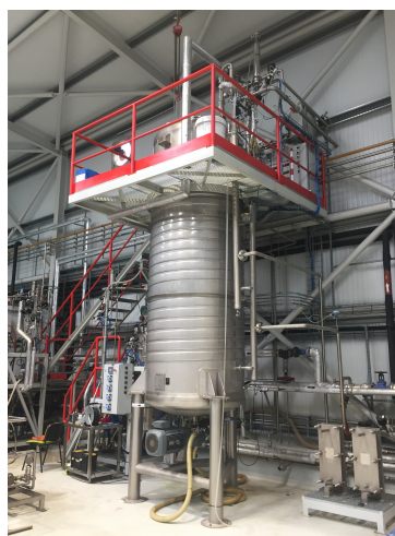
Figure 1.5: Industrial 5000 L fermenter (Allmicroalgae, Pataias, Portugal).
