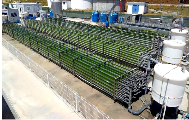
Figure 2.3: Industrial pilot PBRs used in the trials with 2.6 m 3 of working volume (Allmicroalgae, Pataias, Portugal).
